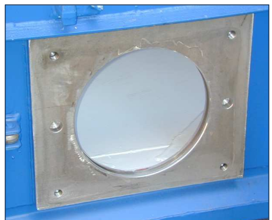
Stainless steel discharge plate DN 250
