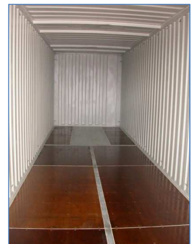
Inside view with plywood floor
